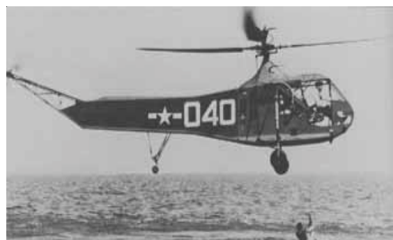
The first helicopter rescue winch is demonstrated in Jamaica Bay off Floyd Bennett Field in 1944. This device proved invaluable in the air - sea rescue role.
